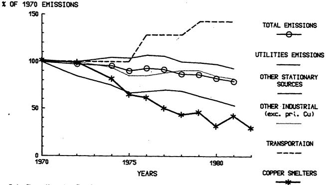
\* Data Shown Here Are For Copper Smelters, But Inclusion of Lead and Zinc Smelters Does Not Haterially Change These Results
